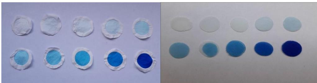
Fig. 1. Photographs of the films deposited on membranes (left) and their composites with PLC (right).
